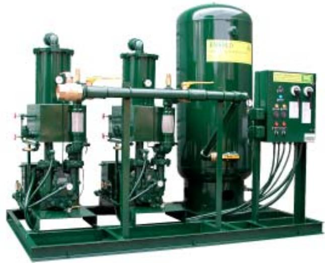
Externally operable circuit breakers with a door interlock, control circuit transformers with fused primary and secondary coils, H-O-A switches, magnetic starters with 3 leg overload protection and reset switches are standard.
