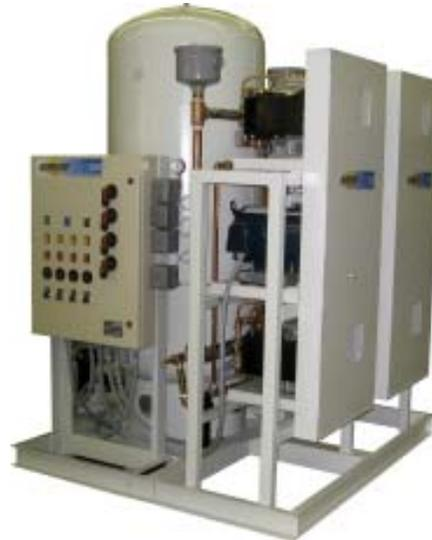
The dryer is designed to provide a maximum dew point below +32°F per NFPA 99. Built-in purge saver control automatically minimizes the amount of purge air to match the variable air flow.
